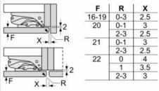
The gap dimensions recommended in the table must be adhered to in order to ensure that appliance doors do not collide with anything when they are opened, and to avoid causing damage to kitchen units.
