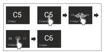
Fig. 21 Example illustration: Switch from C5 to C6.
